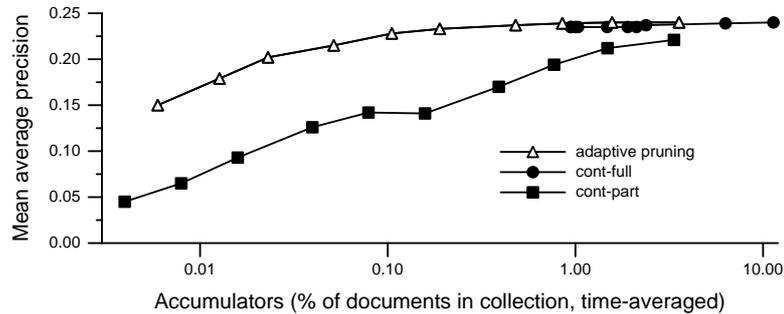
**Fig. 1.** Efficiency-effectiveness tradeoffs in different pruning techniques. The new adaptive pruning approach provides a clearly superior combination of high retrieval effectiveness with accurate management of memory use.
